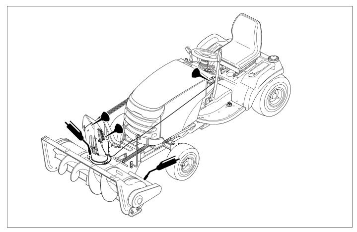
Figure 2. Lubrication Points
